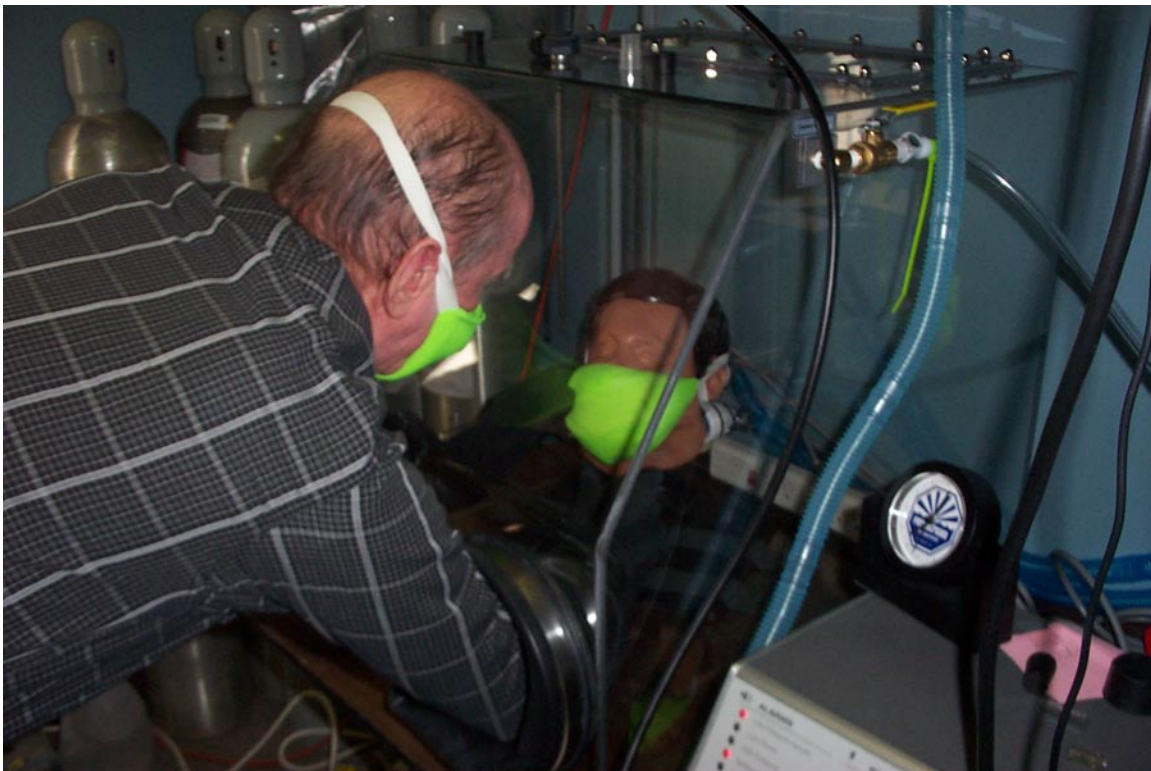
Figure 5. Massaging a Smoke Mask During Active Test
